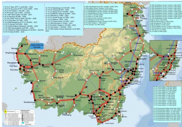
Figure 4 shows Kalimantan's current transmission lines (solid lines) and the planned transmission expansion (dotted line)
